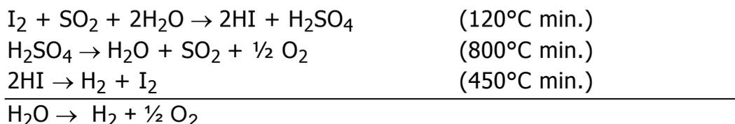
Theoretically, only water and heat need to be added to the cycle. Heat energy enters a thermochemical cycle through one or more endothermic high-temperature chemical reactions. Heat is rejected via exothermic low temperature reactions. All of the reactants, other than water, are regenerated and recycled. Figure 1 shows a schematic of the system.
