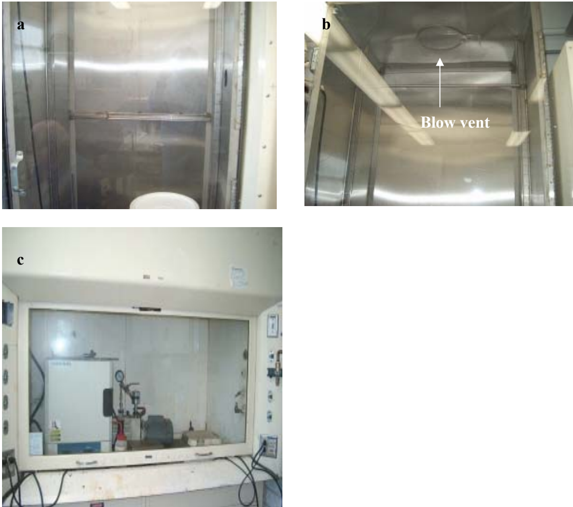
Figure 13. (a) Enclosure for the experimental set up (b) Blow vent at the top of the enclosure and (c) fume hood next to the enclosure for mixing HIX.
