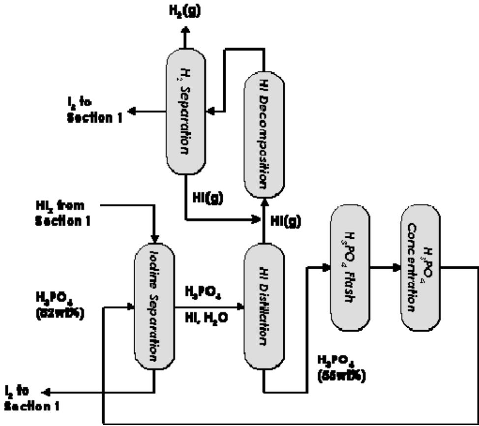
Figure 18. Flowsheet for HI decomposition via extractive distillation.
