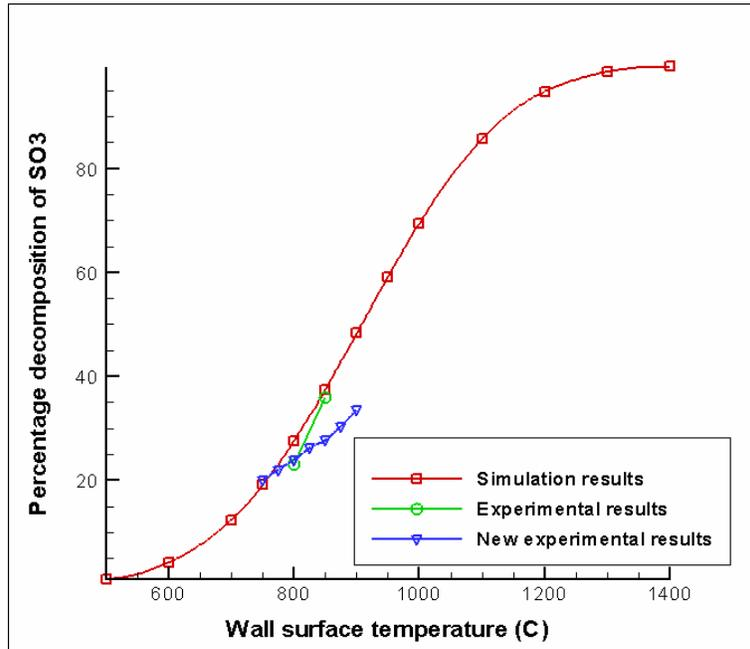
Figure 8. Comparison of percentage decomposition of sulfur trioxide for simulation and experimental results.
