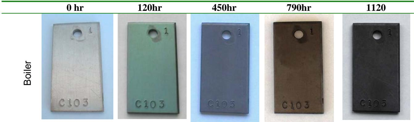
Figure 16. Nb-10Hf coupon tested in  $HI_x$  at the boiler condition
