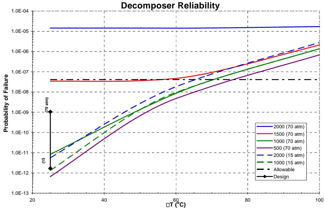
Figure 27. Probability of Failure for Sulfuric Acid Decomposer.
