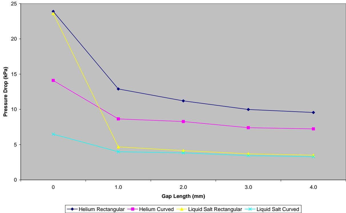
Figure 1. Gap length (mm) vs. pressure drop (kPa) for both He and LS channels.
