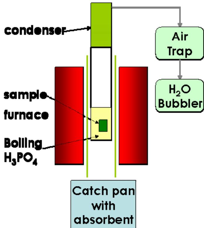
Figure 20. Material test system for the phosphoric acid concentration environment.
