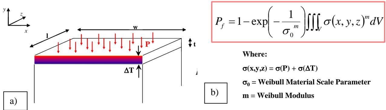
Figure 26. Calculation of the Reliability of the Heat Exchanger Due to Thermo-Mechanical Stresses a) Model, b) Mathematical Formulation.
