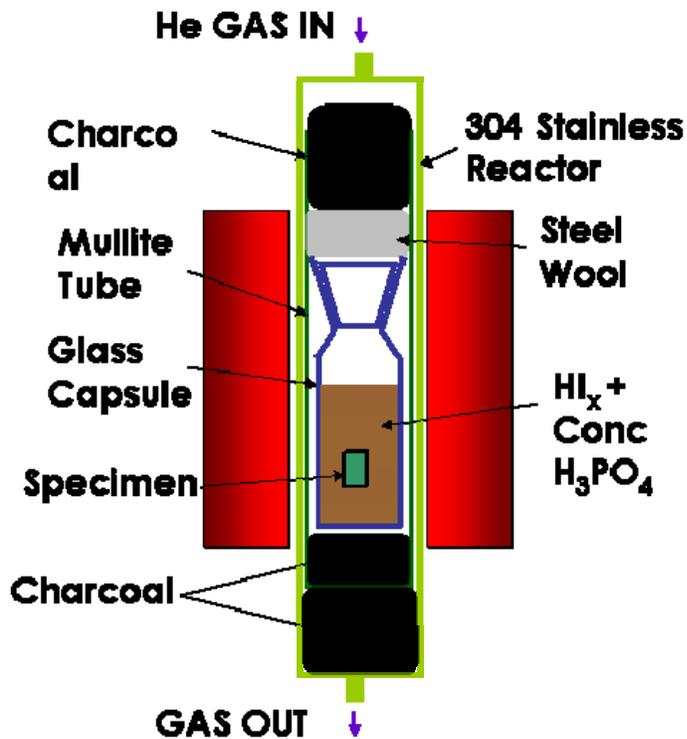
Figure 19. Material immersion test system for the iodine separation environment.
