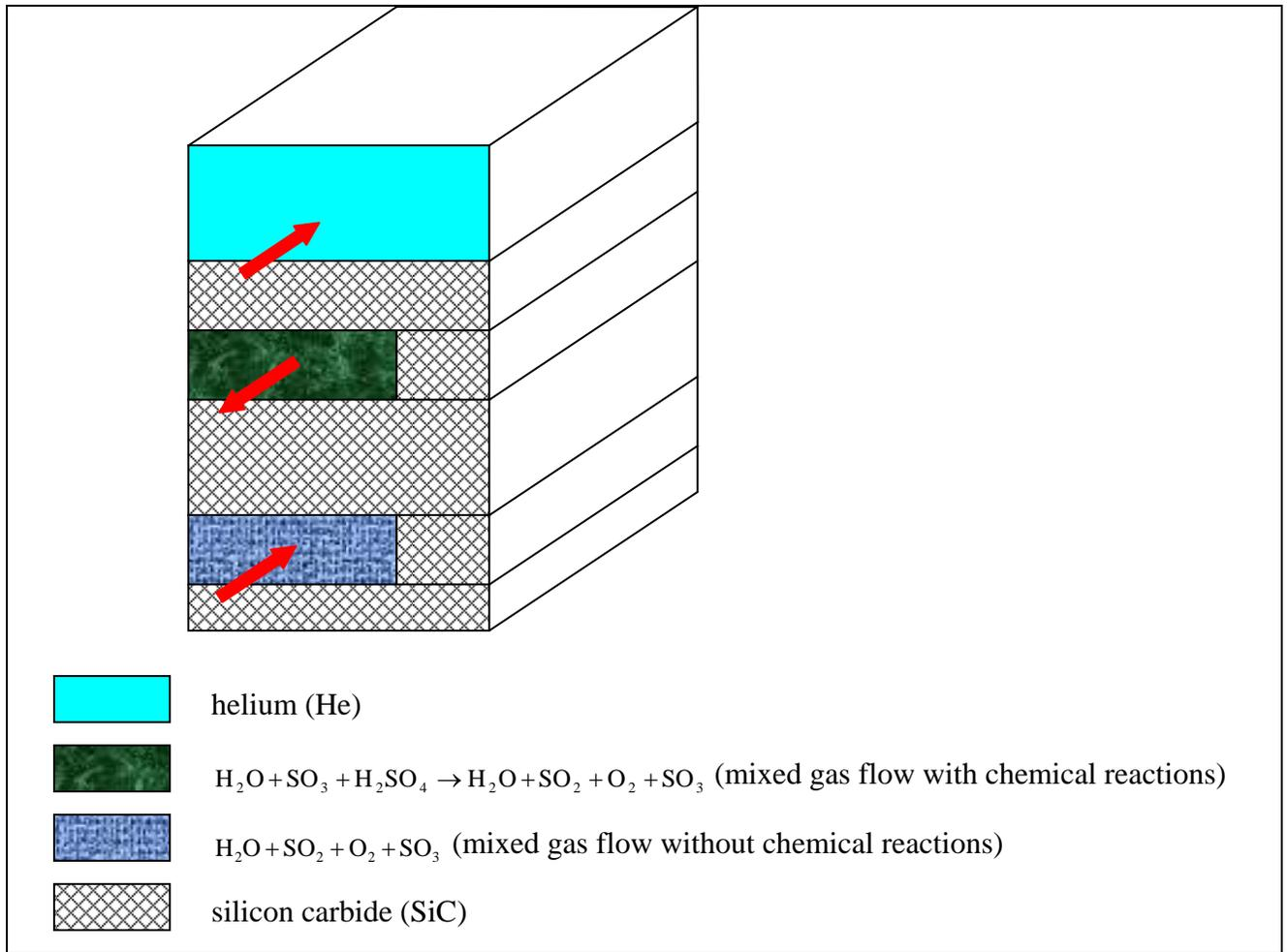
Figure 4. Single channel model of Ceramatec, Inc. high temperature heat exchanger.
