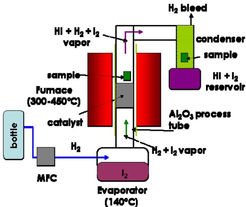
Figure 21. Material test system for the HI gaseous decomposition with flowing gases.
