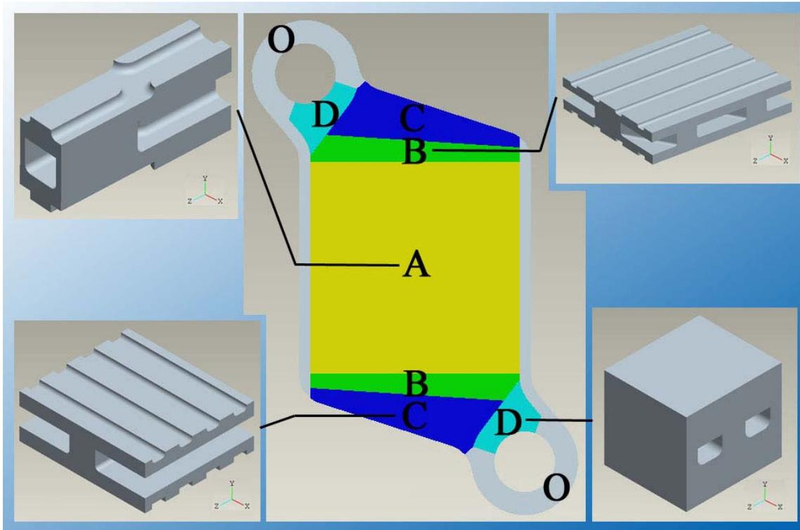
Figure 12. Region division and unit cell models for a HX plate.
