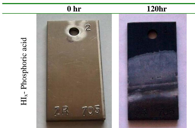
Figure 22. A Zr705 coupon that has undergone immersion coupon testing in the iodine separation environment for 170 hours.
