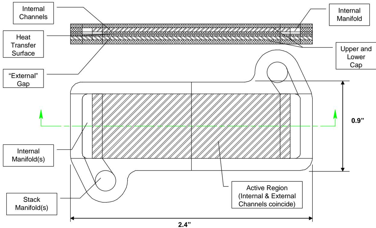
Figure 28. Thermal/Flow Test Coupon (Details of Flow Channels dependent on design Parameters).
