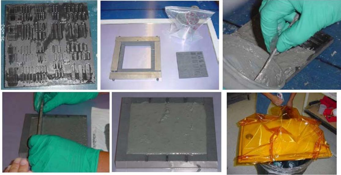
Figure 10. COI tool preparation, lay up and bagging.
