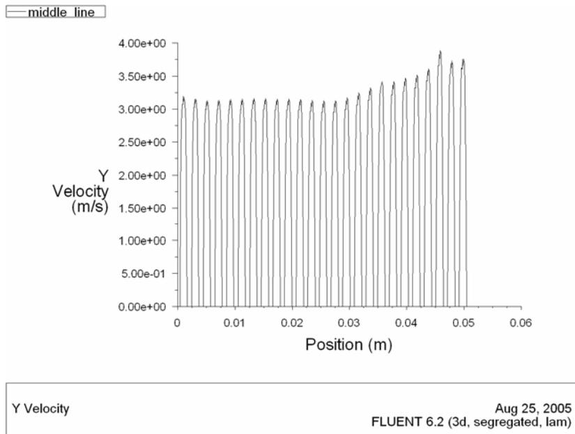
Figure 6. Y- Velocity distribution in the channel centers.
