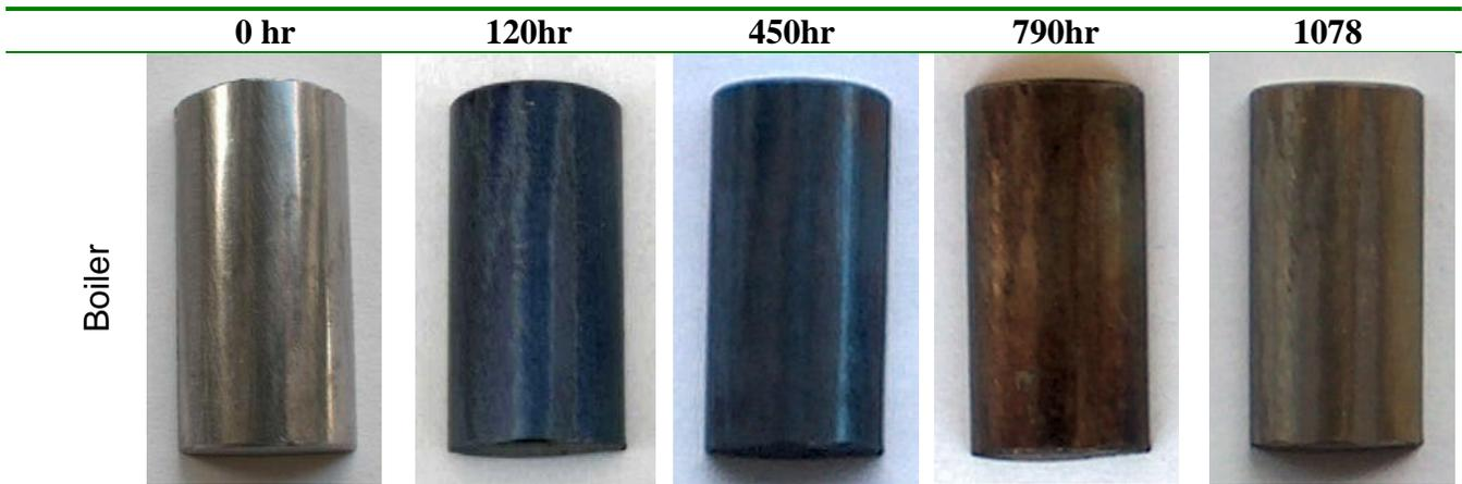
Figure 17. Ta-10W specimen tested in  $HI_x$  at the boiler condition.
