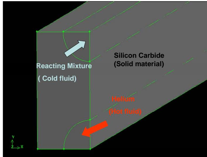
Figure 9. Unit cell of the sulfur trioxide decomposer taken into consideration for grid generation.
