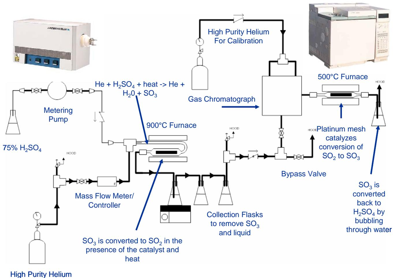
Figure 23. Schematic of Catalyst Effectiveness System.
