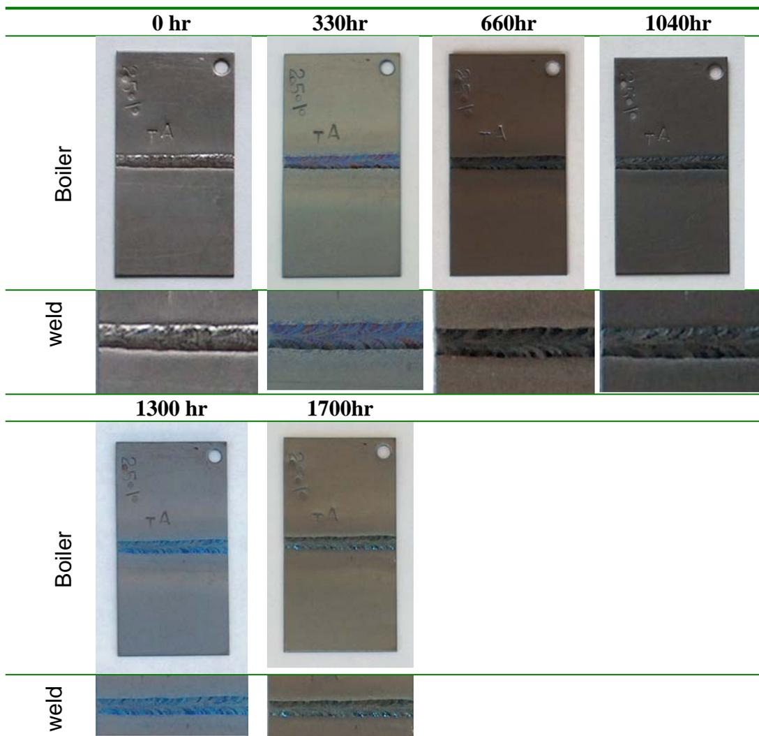
Figure 14. Ta-10W immersion corrosion coupon with an e-beam weld.
