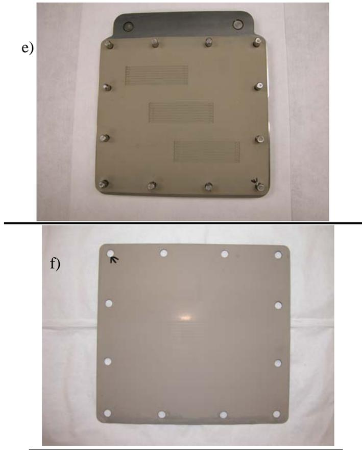
*Figure 29. a) Lamination Press, b) Lamination Die, c) Micro-channel Slots (3-up), d) Manifold Slots (3-up), e) Laminated Wafer (1/2 complete), and f) Laminated Wafer with Enclosed Features.*
