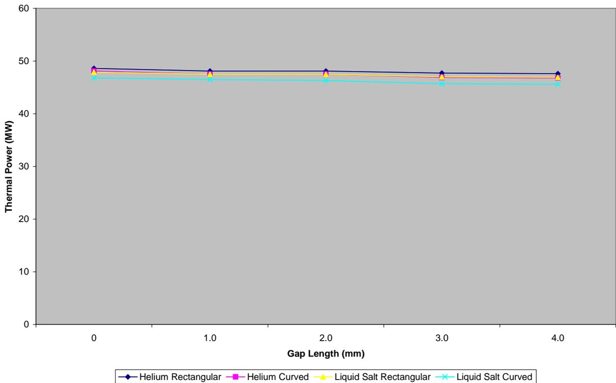
Figure 2. Gap length (mm) vs. thermal power (MW) for both He and LS channels.
