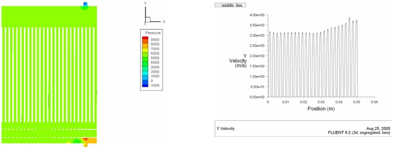
Figure 25. Flow Equilibration Through Optimization of Internal Manifolds.
