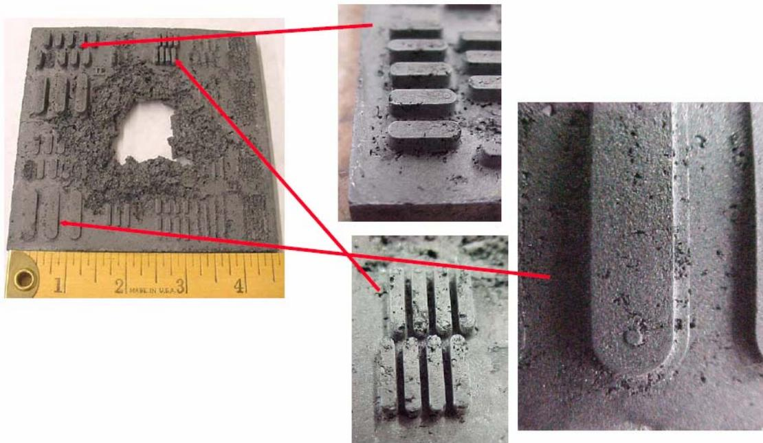
Figure 11. Plate fabricated using new release coating for graphite mold.
