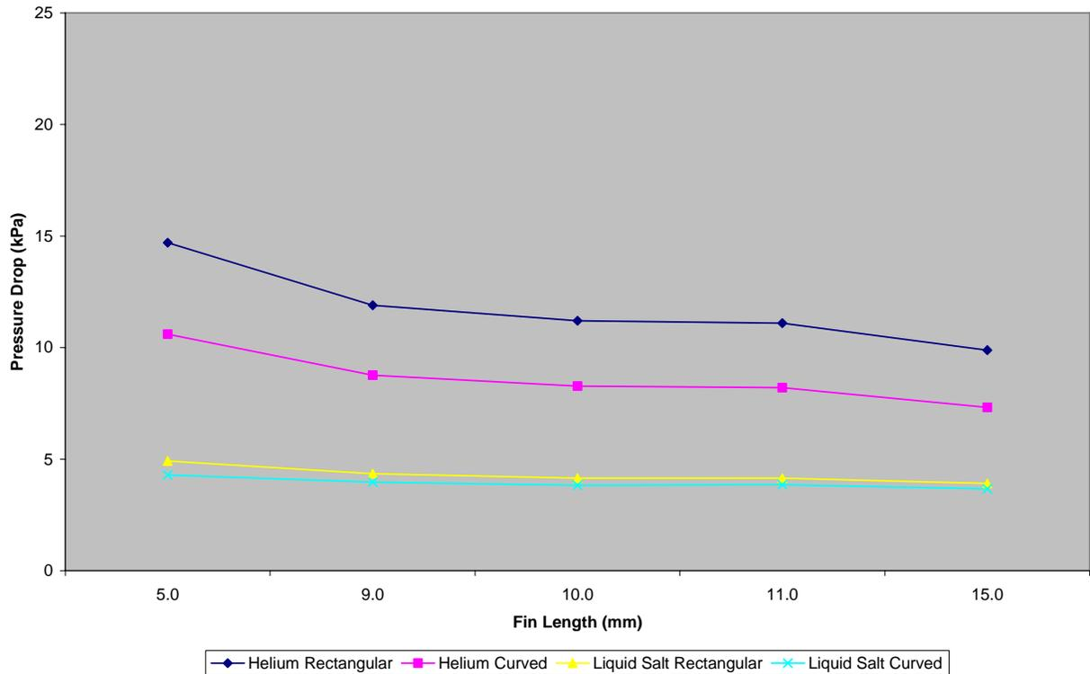
Figure 3. Fin length (mm) vs. pressure drop (kPa) for both He and LS channels.
