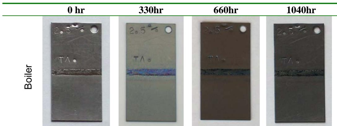
Figure 15. Ta-10W immersion corrosion coupon with an e-beam weld.
