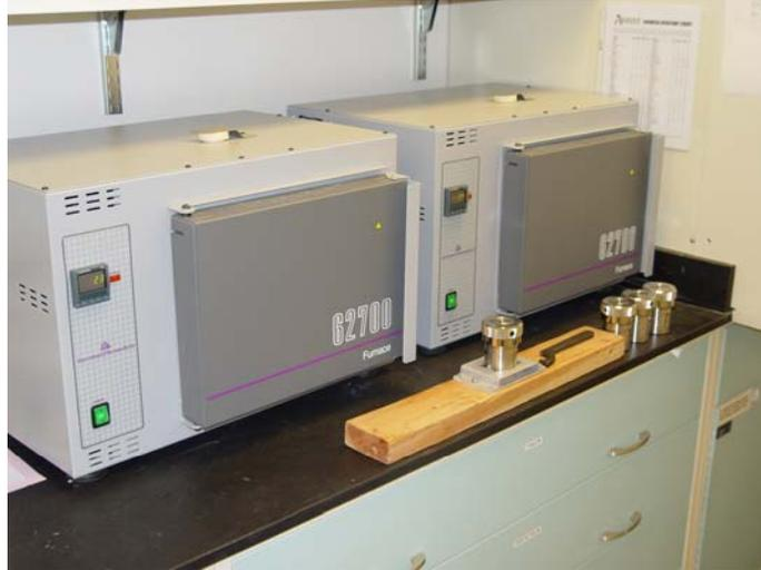
*Figure 8. Two of the muffle furnaces that will be used for the dissolution studies of doped vitrified waste material, along with four acid digestion bombs, sealing bracket, and spanner wrench.*
