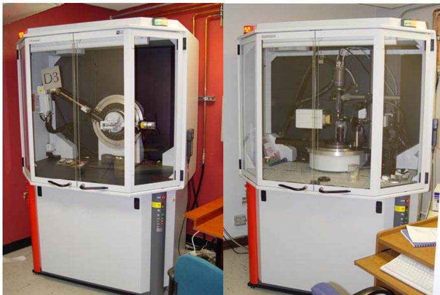
*Figure 11. The newly obtained and installed Bruker D8 Advance X-ray diffractometer (left) and Bruker APEX II single crystal X-ray diffractometer (right).*
