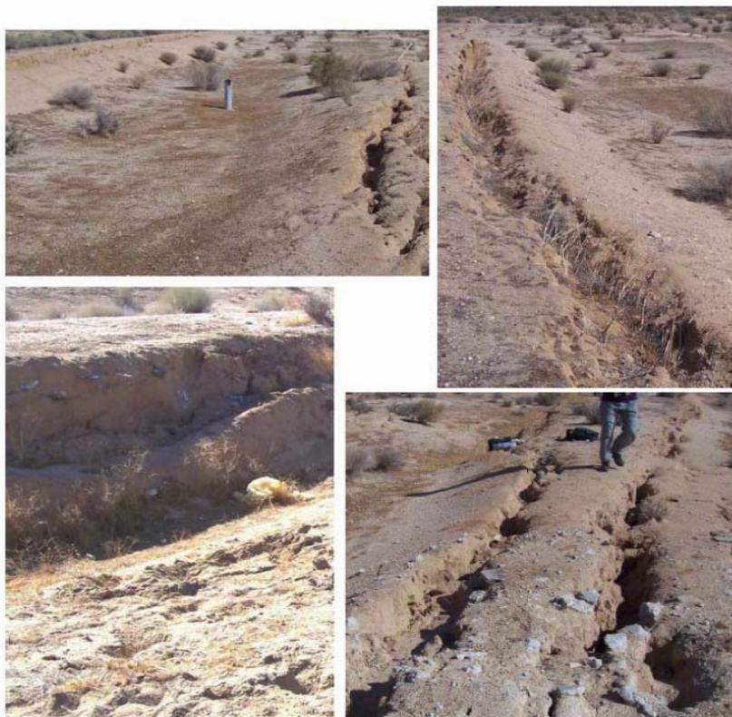
*Figure 1. Differential settlement and tension cracks parallel to waste trenches.*
